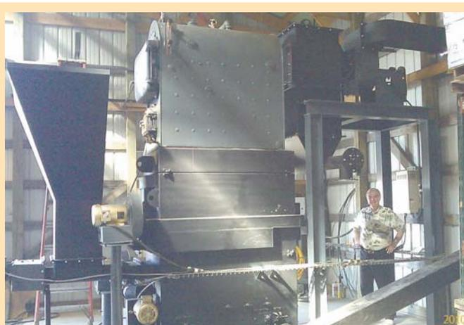
**King Coal biomass furnace is designed as a combustion unit for use with grain driers. The company makes a variety of furnaces, producing one million btu's on up.**
