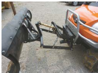
Hitch can also be mounted on front of vehicle and used to support this 3-pt. snowplow.
