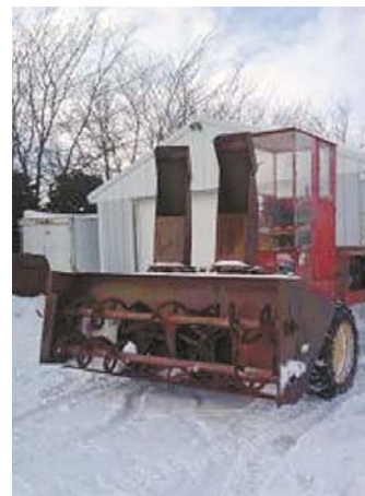
“It’ll turn on a dime and can blow snow out 110 ft.,” says Leon Brech, who built a 9-ft. snowblower and mounted it on a self-propelled swather.
