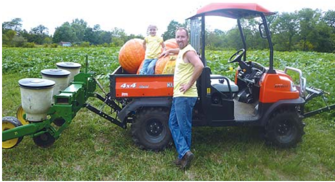
Produce farmer Mark Altemeier uses his Kubota RTV utility vehicle to plant crops, thanks to the add-on 3-pt. hitch he developed.
