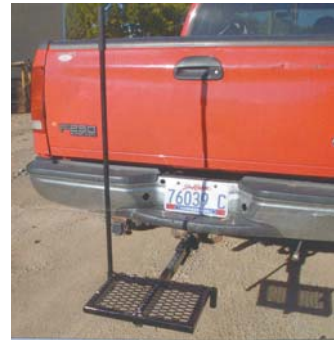
Tailgate step fits into receiver hitch. It comes with a 42-in. long handle that slips into a hole on either side of step.
