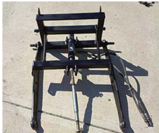
Hitch fastens to utility vehicle’s receiver hitch and comes with 2 bolt-on brackets that hook up to vehicle’s frame.
