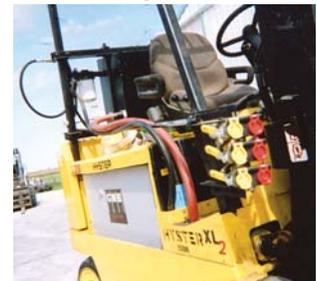
Hydraulic Module On Electric Forklift
