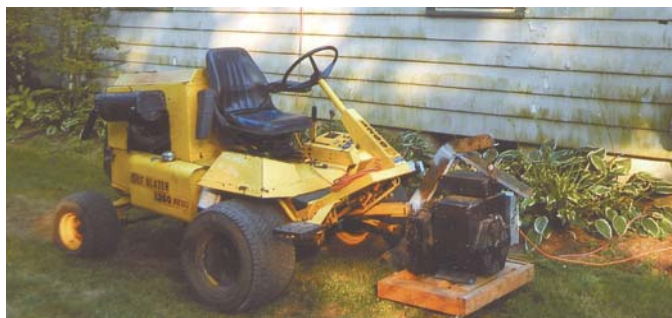
Generator mounts on a homemade wooden dolly and is driven off riding mower's front pto.
