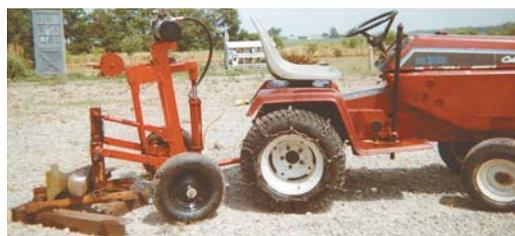
William Hettler's Cub Cadet garden tractor has no hydraulics, so he built this 3-pt. "dolly" for it. Power is provided by a self-contained, 12-volt hydraulic power pack.
