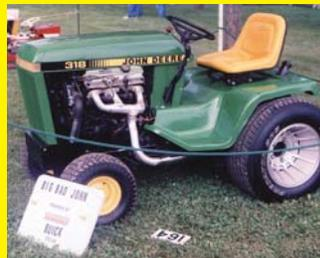
I replaced the original 10 hp engine on my Deere 318 garden tractor with a Buick 6-cyl., fuel-injected engine out of a 1994 Pontiac Bonneville. It has 170 hp so it'll really go. A shaft leads from the engine back to the tractor's hydrostatic transmission. Top speed is only 20 mph but it's really fun to drive.
