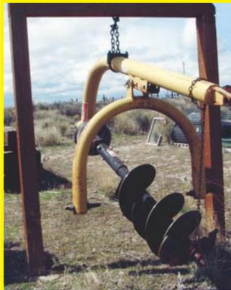
After several strained muscles, I built a posthole auger holder using 4 by 4 posts for the frame. A 3 1/2-in. muffler clamp, with a short loop of chain attached to it, attaches to the frame of the auger. The chain hooks over a clevis hook that's eye-bolted to the top crossbar. Makes hooking and unhooking easy. (Larry Allen, Crane, Ore.)
