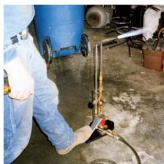
**Brian Johnson, Clearwater, Minn.:** “I made a pedal-operated foot torch using a fuel saver valve block that I bought at a welding supply store. The torch has a pilot light that’s match-flame size. When you step on the pedal, it provides a controlled even heat.
