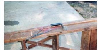
“Carrying a step ladder can be a little awkward. I made it a lot easier by mounting a simple handle on the side of the ladder at the balance point.
