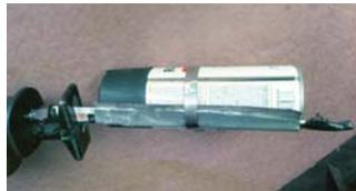
duct tape, use a large hose clamp to attach the aerosol can to the blade, and then run the saw. Works like a charm and is easy on the hands.”
