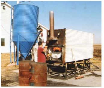
Computerized delivery system feeds corn into stove as needed so it burns at maximum efficiency.
