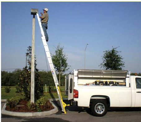
Monkeyrack attaches to a standard 2-in. receiver hitch to hold ladders up to 20 ft. tall (left). Bottom of ladder rests on ground.
