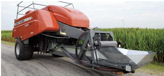
**Bolt-on unit allows combine to pull baler, harvesting grain and crop residue at same time. Enclosed conveyor delivers material to baler.**
