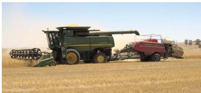
**A hydraulic motor, powered by an independent hydraulic pump on combine, drives baler.**
