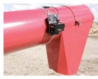
Magnetic camera system helps operator on ground line up auger with opening on top of grain bin.
