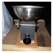
Norm Erickson has developed machines to husk, sort and crack hazelnuts, and then clean and size the kernels. Mechanical hammer (left) cracks nuts against an anvil.
