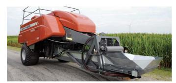
Bolt-on unit allows combine to pull baler, harvesting grain and crop residue at same A hydraulic motor, powered by an independent hydraulic pump on combine, drives baler.
