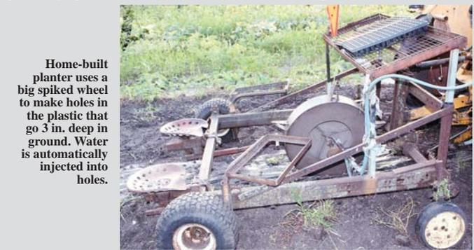
Home-built planter uses a big spiked wheel to make holes in the plastic that go 3 in. deep in ground. Water is automatically injected into holes.
