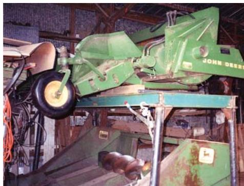
Double stacked combine headers free up storage space in Oldenberg's machine shed. An adapter he made to fit his tractor loader hooks up to headers, making them easy to move around.
