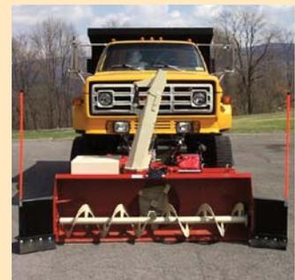
Snow Vac snowblower can be moved from tractor to truck and back in minutes when both vehicles are equipped with quick-attach systems.
