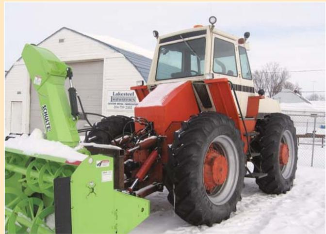
To clear out snow, Derek Jenkins reversed the cab on a Case 4490 tractor and mounted a 110-in. Schulte snowblower on front.
