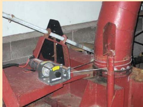
A small electric winch, operated by a push button controller mounted on tractor fender, is used to rotate the chute on 3-pt. mounted snowblower.
