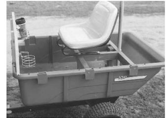
**Seat is off a Deere 212 riding mower and mounts on spring-loaded brackets that are lag bolted to a wooden frame.**
