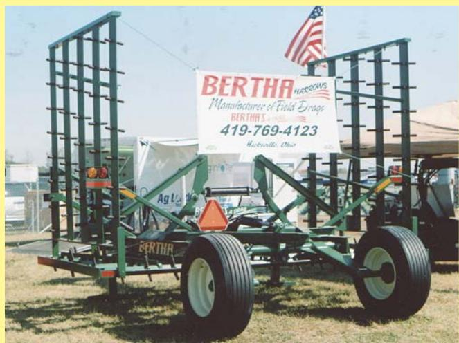
**The front and rear half of the Bertha harrow can be hydraulically raised or lowered to prevent gouging and to allow trash to flow through.**
