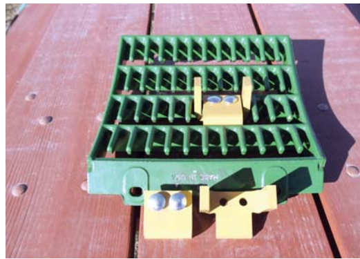
CM Welding’s concave grate replaces the rear concave in Deere STS rotors. It’s fitted with “disrupter” add-ons to reduce grain loss.
