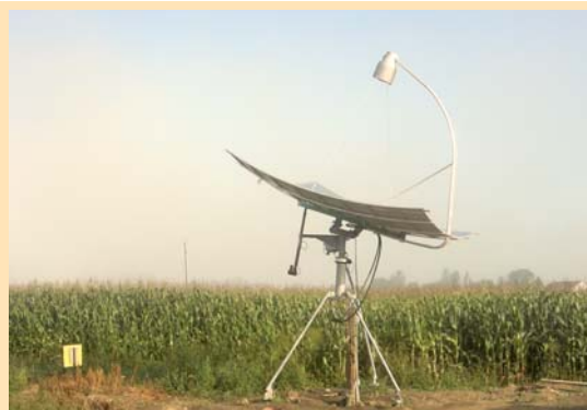
Solar “concentrator” uses curved panels to capture the sun’s rays at a precise focal point to generate heat.
