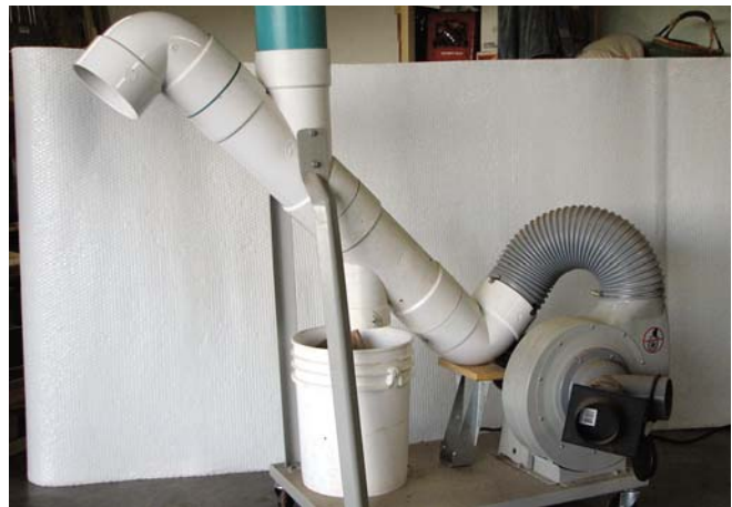
Aspirator uses a high-speed fan to remove trash, which is blown out an exhaust pipe.
