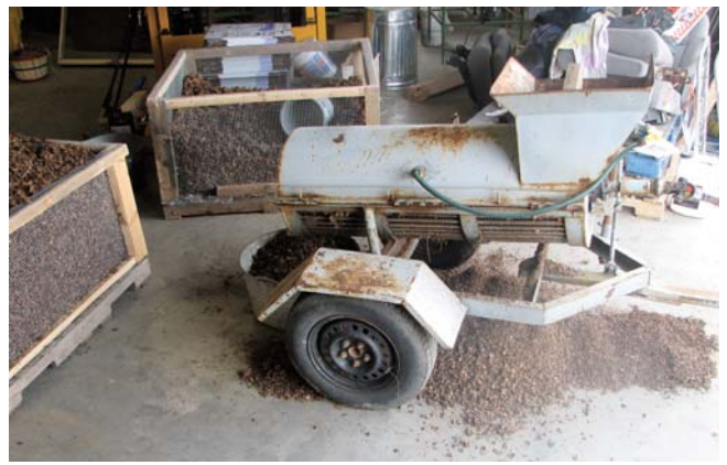
Home-built husker – a modified walnut huller - can handle 2,000 lbs. of nuts per hour.
