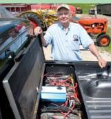
Located behind the pickup cab, the battery case comes with 10 deep cell, lead acid batteries which recharge in just 4 hours.
