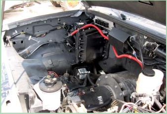
With no engine there's a lot of room under the hood. Photo shows 100V, DC electric motor, which drives a 5-speed manual transmission using Mag-Trans technology.
