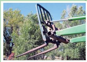
Salvaged from an old electrical warehouse forklift, the forklift mast pins to the front-end loader on Shearer's Deere 3020 tractor.
