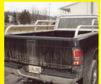
firewood. I made the rack higher in front so I can haul more wood. I also use the pickup to haul my ATV and canoe so I welded 8 tie-down lugs onto the rack.
