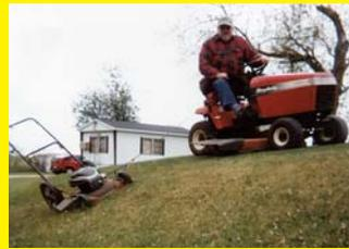
to cut grass on steep hillsides. These photos do a better job of showing what I did. I bolted a boat winch onto the rear fender of the tractor and bolted safety belt anchors to one side of the mower, on front and back. Then I made up a 15-in. long chain with a hook at both ends, and attached each end to an anchor.
