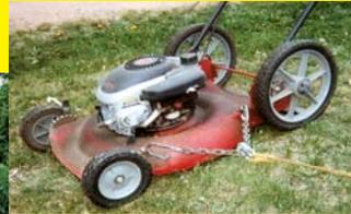
I drive the tractor along the top of the hillside so the mower follows along below me. When I reach the other end, I make a U turn to bring the mower back up. Then I crank the winch again to lower the mower and make another pass.
