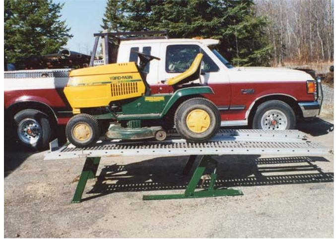
Once the riding mower reaches a tipping point, deck tilts back to a horizontal position.
