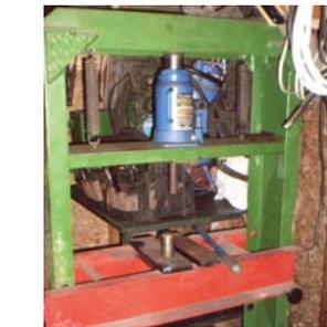
press had three short, thin screw-in handles that stuck out at an angle and provided no leverage. The handles pulled hard, and I couldn’t keep them tight because the threads often stripped where the handles were screwed on.
