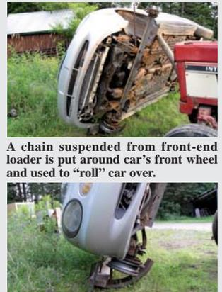
A chain suspended from front-end loader is put around car’s front wheel and used to “roll” car over.
