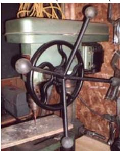
handles with a big 12-in. dia. wheel that came off a valve. The wheel has four 1 1/2-in. dia. metal handles welded on with knobs, scrounged from hydraulic control levers, friction-fitted to the ends. When using small bits with the drill press I just hold onto the wheel, but when using large bits I hold onto the handles to get more leverage. The improvement in the way my drill press handles now is beyond belief.”
