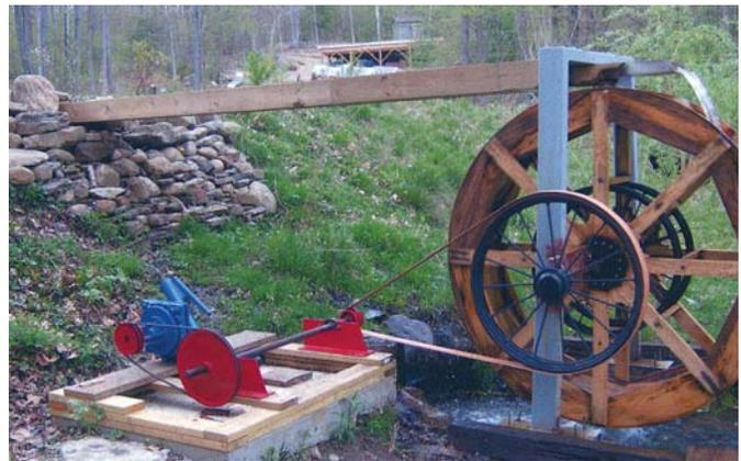
Water wheel makes electricity by belt-driving a 100-watt generator.
