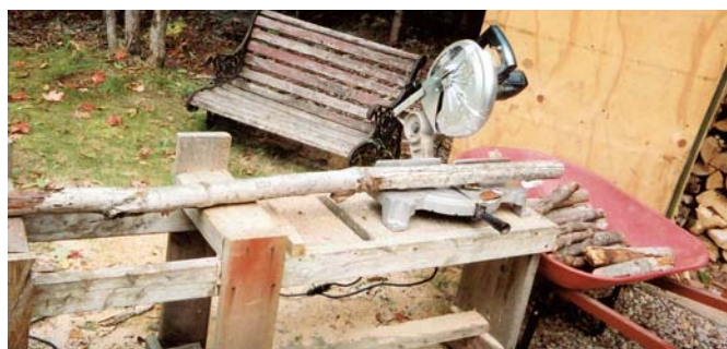
Ken Gustafson uses an electric-operated, 10-in. miter saw to cut small chunks of firewood.
