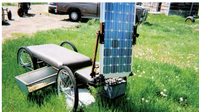
Battery-powered, crop-picking cart is equipped with a solar-powered charger.
