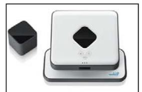
GPS-like guidance system tracks where robotic floor cleaner goes.
