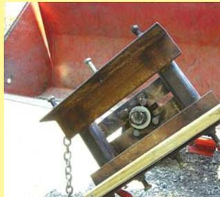
Double-nutted, 1-in. dia. threaded rod tightens device to bucket lip (left). A post holder with angle iron sides is then attached to threaded rod.
