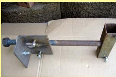
Dan Servideo recently used his loader-mounted post clamping device to pick up and place 8 5/8-in. sq. pressure-treated posts.
