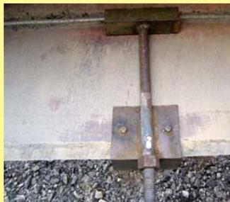
Double-nutted, 1-in. dia. threaded rod tightens device to bucket lip (left). A post holder with angle iron sides is then attached to threaded rod.
