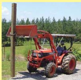
Dan Servideo recently used his loader-mounted post clamping device to pick up and place 8 5/8-in. sq. pressure-treated posts.
