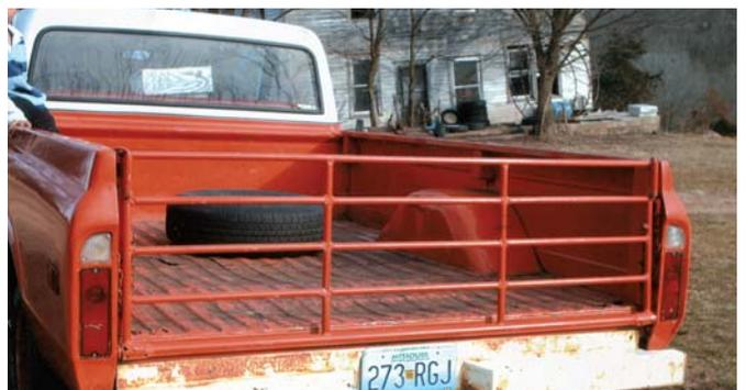
Dale Herigon used old galvanized water pipe to make this new tailgate for his pickup.
