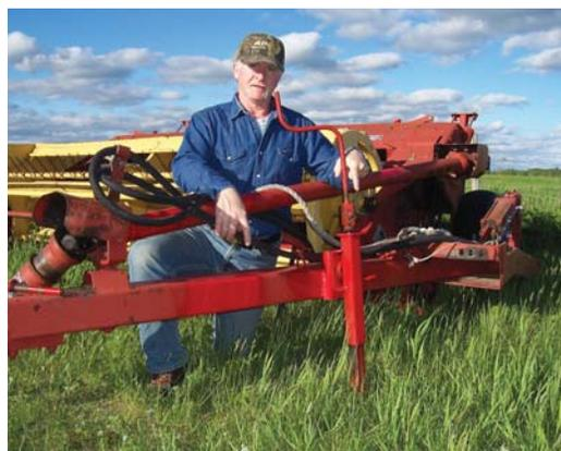
The lift jack on Bruce McNamara's haybine was causing the jack to cut into tractor's rear tire on turns. So he cut off the jack assembly and moved it back 16 in.
