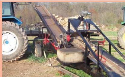
Hydraulically-controlled firewood processor loads split wood into a truck or wagon.
