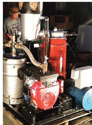
All kinds of waste can be used to power the new "Power Pallet". A gasifier control unit automatically adjusts the fuel-air mix for the material being burned.
