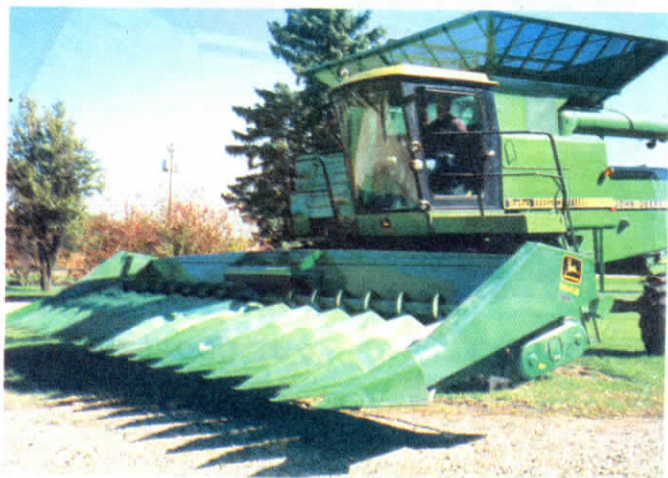
Ricke merged two Deere 8-row corn heads to build the 16-row, 20-in. corn head. He also mounted a 200-bu. extension on top of combine's 250-bu. factory tank.
