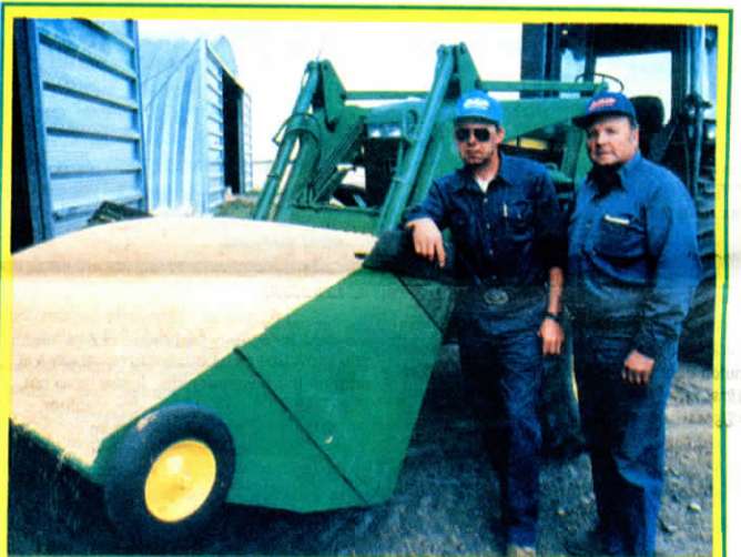
The Helgasons turned an 8-yard bucket from a damaged pull-type scraper into a 52-bu., 2-wheel "floating" grain bucket on their Deere 265 front-end loader.
