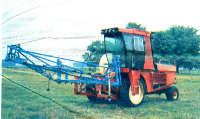
Berry mounted 500-gal. tank and cradle on side of power unit and fitted 60-ft. sprayer boom to front toolbar holder.
