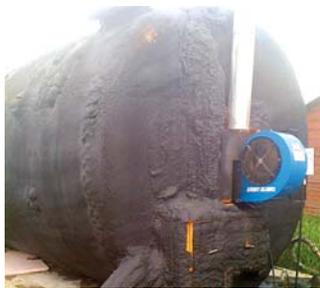
Burner was built out of 2 large underground fuel tanks.
