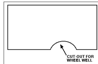
Sideboards consist of 4 by 8 plywood sheets with cut-outs for the wheel wells.
