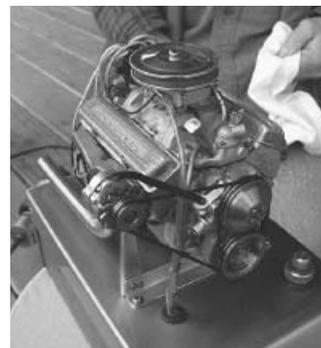
Jim Moyer made this working 1/6-scale Chevy 327 cu. in. V-8 engine.
