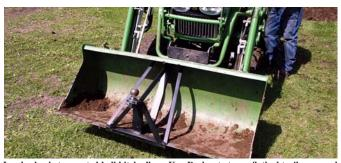
Loader bucket-mounted ball hitch allows Ken Dreher to tow a flatbed trailer around with his tractor.
