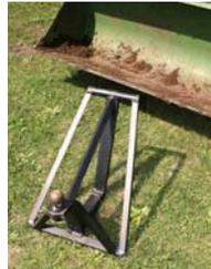
Slip-in hitch requires no modification to bucket. It can be removed simply by tipping bucket toward the ground.
