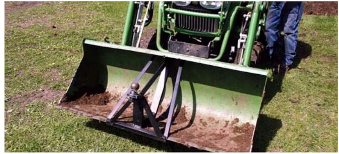
Loader bucket-mounted ball hitch allows Ken Dreher to tow a flatbed trailer around with his tractor.
