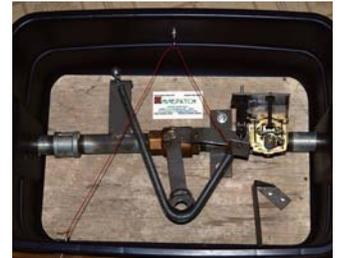
When water pressure drops, a trigger-release spring closes a valve and flips up the spring-loaded stick like a tip-up.
