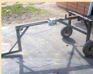
Log skidder’s wheels came from an old trailer, and the heavy-duty winch was purchased new for about \$75.
