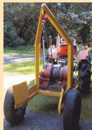
Skidder is equipped with a heavy-duty tow truck winch that’s belt-driven by a Briggs & Stratton 6 1/2 hp engine.
