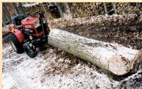
Dan Jacobson’s home-built log skidder mounts on front of his Yanmar 18 hp garden tractor.
