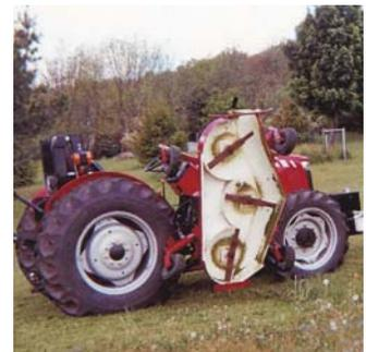
**An ATV winch that operates off the tractor battery is used to fold the mower upright for transport.**
