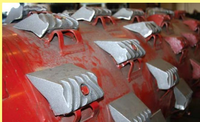
High performance thresh bars are designed for AFX/specialty rotors in Case IH combines. "They work especially well in hard threshing crops," says inventor Ron Kile.
