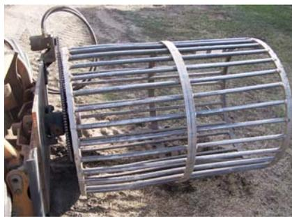
Rock picker attaches to front of skid steer loader and tilts down to pick up rocks. After it's tilted back up, unit rotates to spin off dirt and debris.
