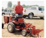
Peternell built this 3-wheeled trailing plow equipped with a 12-in. moldboard and a 12-in. coulter.
