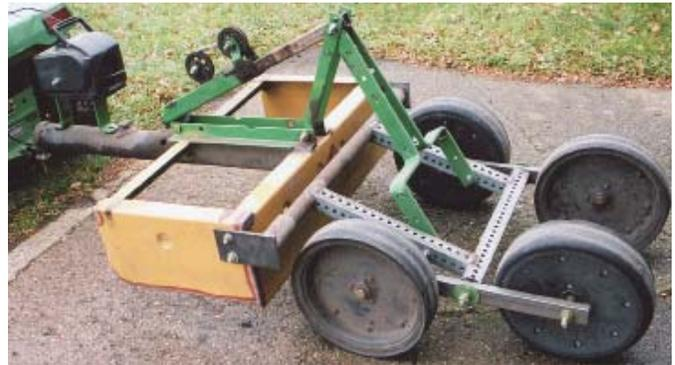
Elroy Lindaas built this 4-ft. wide box scraper using 4 discarded closing wheels off an old air seeder.
