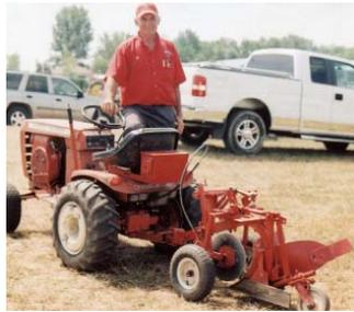
Peternell built this 3-wheeled trailing plow equipped with a 12-in. moldboard and a 12-in. coulters.
