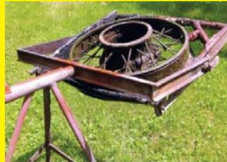
Thanks for the story on my wheel painting tool (Vol. 34, No. 4). Here's another photo that shows the unit holding the wheel. The wheel is held in the center where the tube goes. The wheel can be turned in any direction so the paint will hit it. I've painted at least 2,000 to 3,000 wheels with this tool. It's inexpensive and simple to build. (**Loren Smith, 16033 County 5, Spring Valley, Minn. 55975 ph 507 421-9996**)
