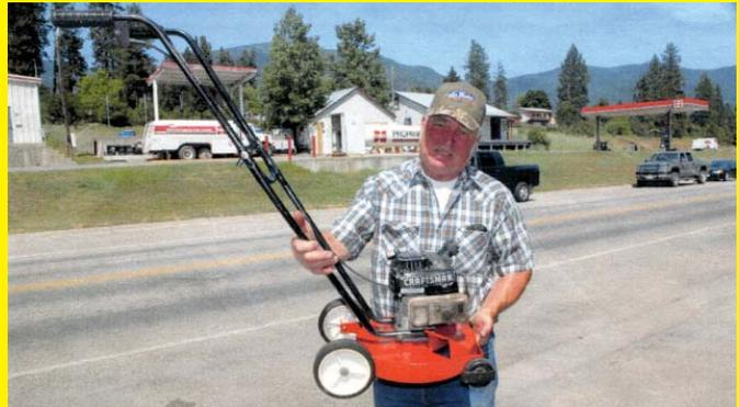
This is a 12-in. lawn mower I made from scratch because I couldn't find a small mower for use around my garden and fence. The engine came from a small rotor tiller that I found in the trash.
