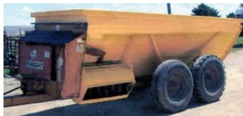
Before and after photos of the Knight manure spreader rebuilt by Al Kilburg. Spreader still has the original wheels, axles and drive mechanism.
