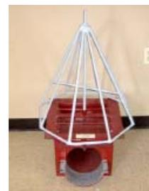
A 3-in. spike on top of tripod breaks the crust, and unit’s sloping sides push it off to the side so grain can flow through.
