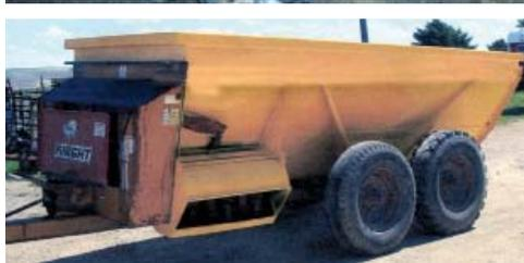
Before and after photos of the Knight manure spreader rebuilt by Al Kilburg. Spreader still has the original wheels, axles and drive mechanism.
