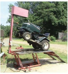
Home-built tractor service lift is made from a Harbor Freight manuallyoperated motorcycle lift table.
