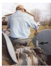
PVC pliers holder bolts onto tractor fend-Whenever I sit down on the tractor seat I just drop the pliers into the holder,' savs David Novotny.
