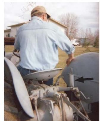
PVC pliers holder bolts onto tractor fender. "Whenever I sit down on the tractor seat I just drop the pliers into the holder," says David Novotny.
