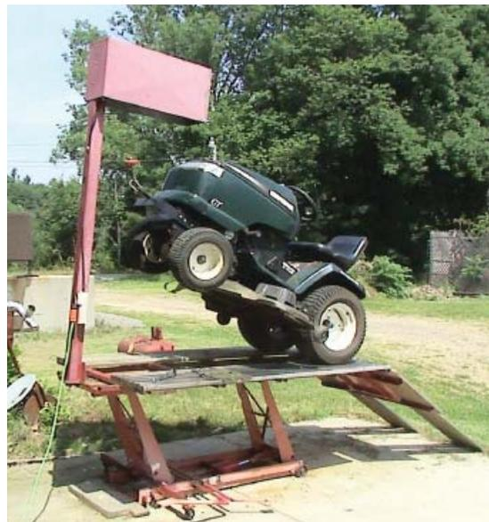
Home-built tractor service lift is made from a Harbor Freight manually-operated motorcycle lift table.
