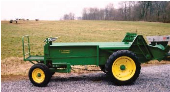
Ground-driven manure spreader is available with 2 or 4 steel or rubber wheels. The 4-wheel model has a front-end steering axle.
