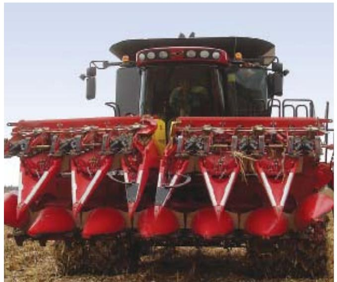
The new Capello corn head can be fitted to most combine brands and is available in a full range of models, either rigid or folding. Chopping rotors are available on all models except the 18-row.
