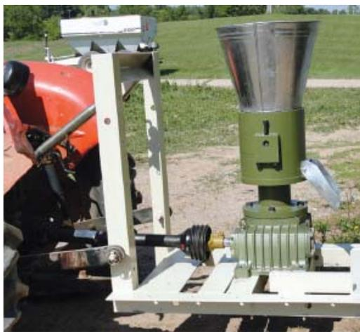
Pto-powered pelletizer has a heavier-duty gearbox that’ll stand up to increased pellet-making torque, says the company.
