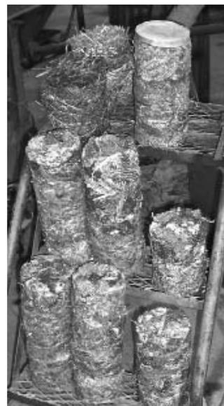
Large-scale pelletizer presses switchgrass or corn stalks into 6-in. dia. “pellets”.
