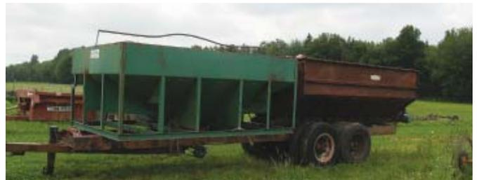
Gabriel Verleun made this 700-bu. grain trailer by mounting a 12-ft. fertilizer wagon on front of a truck chassis, then adding a 14-ft. potato wagon behind it.
