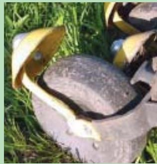
Scraper is offset 1 in. from center of packer wheel (above). Inventor Gerard Devloo pressed the scrapers out of flat 8-in. dia. metal discs in his shop (above right) and then paints them Deere yellow.
