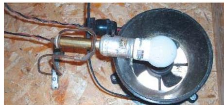
Brian LaDuke used a photocell, old computer fan and small fluorescent bulb to build this mosquito “trap”.
