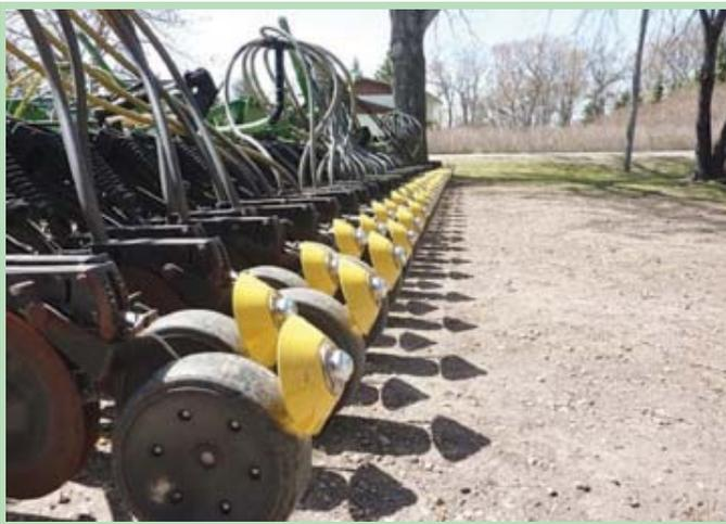
Rotating “cup scrapers” bolt onto air seeder’s packer wheel mounting arm at about a 45 degree angle to keep mud from building up.
