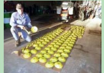
the packer wheel and its outside edges. I tried using a straight scraper blade, but a straight blade can’t follow the contour of the packer wheel like a curved one can. Also, stationary blades wear out quicker and are more likely to plug up with mud. After 3,000 acres my cup scrapers show hardly any wear at all.
