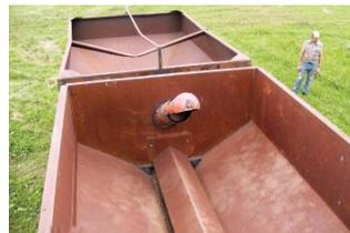
An auger in front wagon unloads grain into back wagon (left). Back wagon unloads via a chain-type conveyor.
