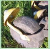
Scraper is offset 1 in. from center of packer wheel (above). Inventor Gerard Devloo pressed the scrapers out of flat 8-in. dia. metal discs in his shop (above right) and then paints them Deere yellow.
